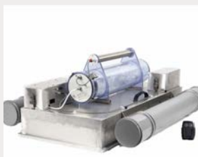
Fig 1 Figure 1 - Equipment used for determining odour emission rate from passive area sources.
