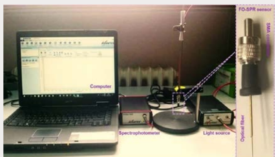
Fig 1. The developed Fiber Optic Surface Plasmon Resonance (FO-SPR) detection system. On the left is an enlarged image of the FO-SPR sensor fixed in an SMA connector. This system comprises the following components: (1) a halogen light source, (2) a UV-Vis spectrophotometer, and (3) an interchangeable FO-SPR sensor inserted into an SMA-type connector.
