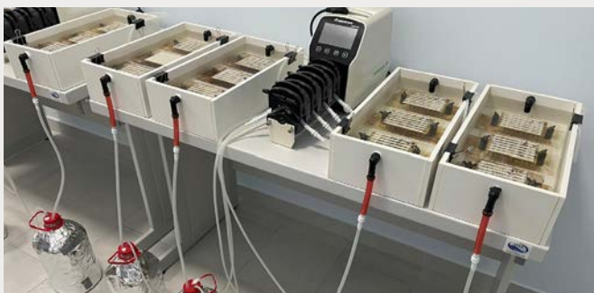
Fig 2. Laboratory artificial lotic systems used to study biodiversity changes caused by pollution. Each artificial system contains glass slides covered with bacterial biofilm and is filled with constantly recirculated sterilized river water using a peristaltic pump.
