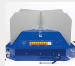
Fig 1 Figure 1 - Equipment used for determining odour emission rate from passive area sources.
