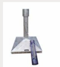
Fig 1 Figure 1 - Equipment used for determining odour emission rate from passive area sources.
